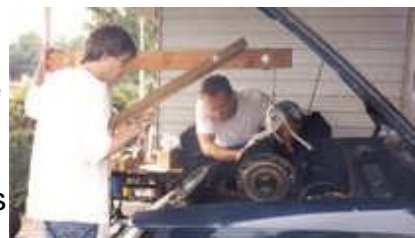
Lowering the completed motor assembly
