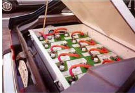
Rear battery box installed
