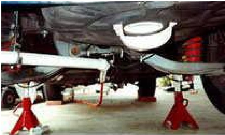
Underside showing conduit, battery box vent and air bags installed.
