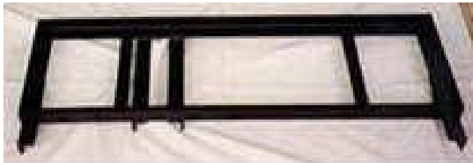
Front rack which will support three batteries, the motor and controller
