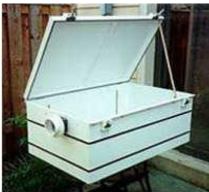
Rear battery box
